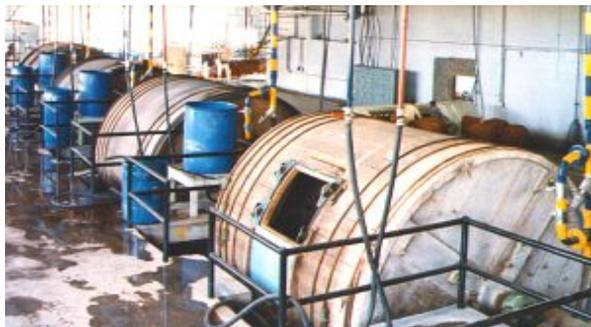
**Figure 1- Dry/Wet Process Drum**
