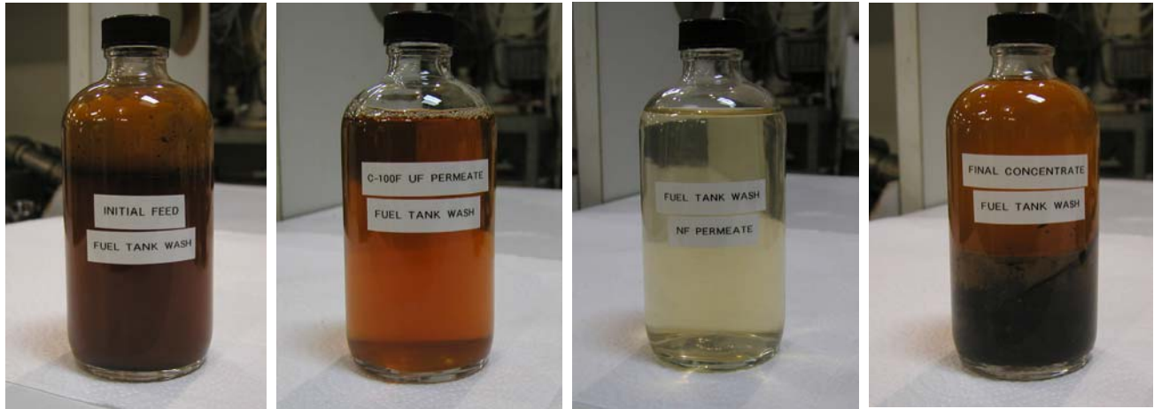
Grab Samples from V-diamond-SEP filtration of Tank Wash Water. The center two pictures show the difference between Ultrafiltration Permeate and Nanofiltration Permeate
