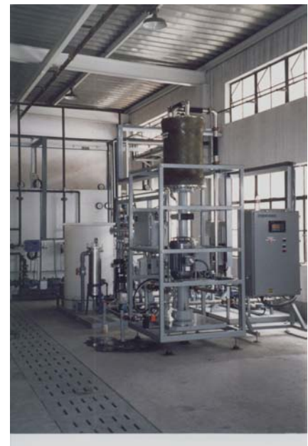
V⇄SEP NF Membrane System installed at a major manufacturing facility for oily water filtration.
