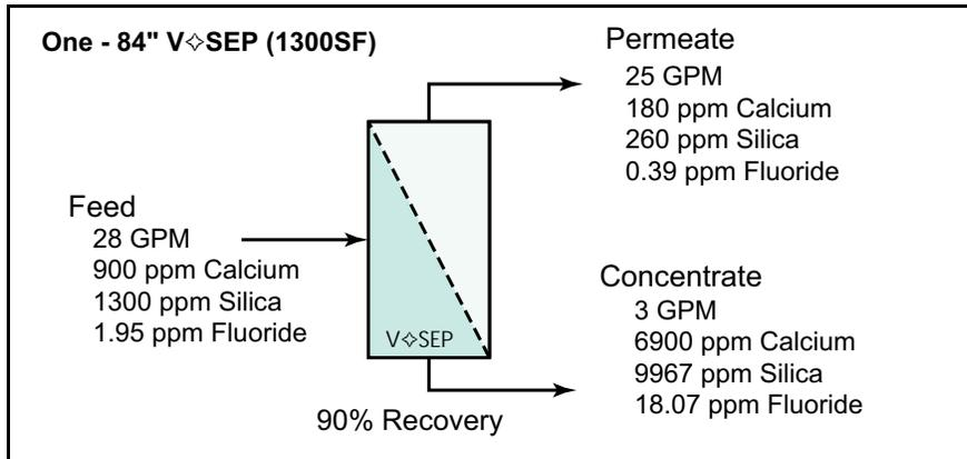
(Programmable Logic Controller) which monitors pressure, flow rate, and frequency. It also provides the safety in operation by monitoring conditions and initiating an alarm shut down should some configurable parameters be reached. The controls include the PLC, Operator display, and process instrumentation. The Filter Pack is mounted on the V◇SEP base unit and contains about 1300 SF, (120m<sup>2</sup>), of membrane area and is constructed out of high temperature materials.
