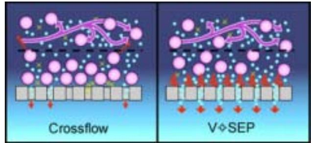
filtrate from the feed material. The liquid fertilizer can be filtered in a single pass filtration using V◇SEP. Other methods like filter presses are done in batch mode with operators opening and cleaning the filter cake on a regular basis. V◇SEP is a continuous automated process requiring very little operator attendance.
