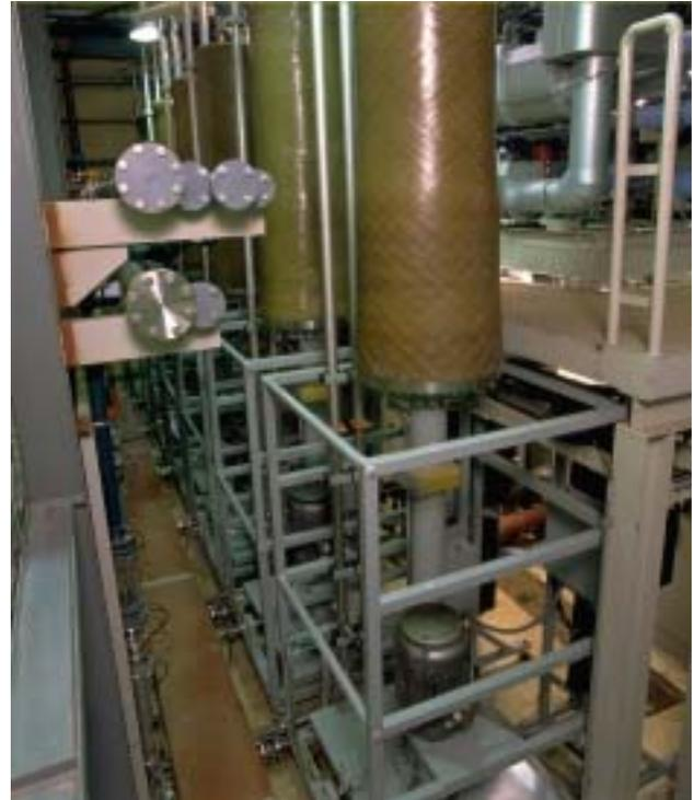
V◇SEP - Vibrating Membrane System suitable for Phosphate Acids & Fertilizers
