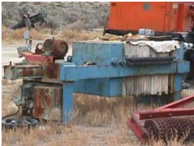
Filter Press is the conventional technology for Phosphoric Clarification
