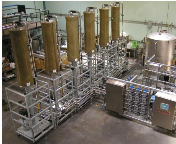
for membrane oxidation protection along with anti-scalant and pH adjustment to maximize flux and minimize the cleaning frequency. The system produces permeate that is blended with other waste streams to improve their collective quality before being discharged.
