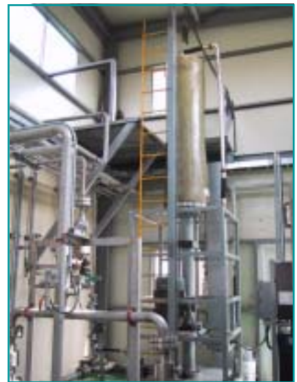
Kimhae Korea - V◇SEP New Logic's patented V◇SEP equipped with 1300 SF (120m 2 ) Reverse Osmosis membrane for the treatment of Hog Manure after a Sequencing Batch Bioreactor
