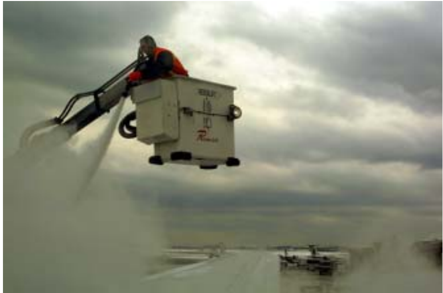
ADF (Aircraft Deicing Fluid) is applied hot by high pressure washing to melt and remove ice, snow, and frost from the airplane surfaces
