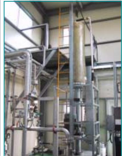
**New Logic's patented V◇SEP equipped with 1300 SF (120m<sup>2</sup>) membrane for the treatment of Chemical Processing dewatering**
