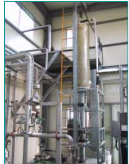
New Logic's patented V◇SEP equipped with 1300 SF (120m 2 ) membrane for the treatment of Chemical Processing dewatering
