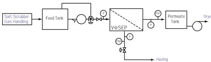
Figure 3: Simplified flow diagram of industrial unit.
