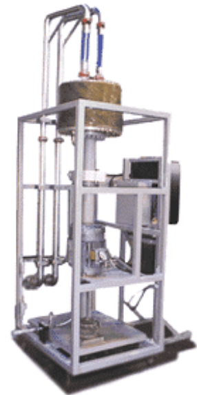
Figure 4: Industrial unit photo. This photo shows the installed filter pack that is 15” tall.
