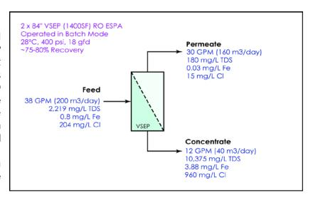
The VSEP system with the RO membrane is producing 42,000 gallons per day (160 m3/day) of additional treated water that would have been disposed of. This reduced the amount of water that needed to be extracted from the groundwater wells.
