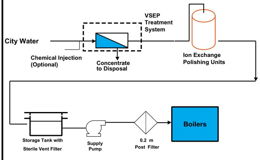
Several technologies are currently being used for boiler feed water treatment. Table 1 presents a summary of the benefits of VSEP when compared to selected competitive technologies such as chemical addition/clarifier systems and cross flow filtration/ spiral membranes. VSEP offers significant advantages over these technologies, as presented in Table 1.
