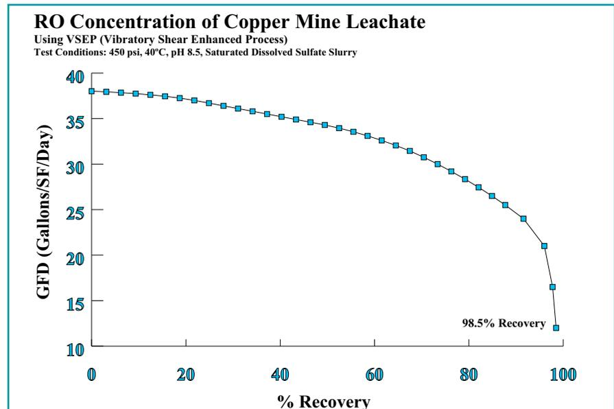
30 GFD (Gallons per Square Foot per Day). System throughput is also a function of the extent to which the feed is concentrated.
