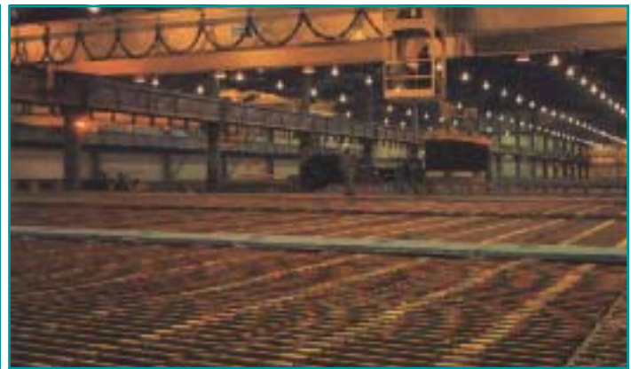
“Electrowinning” - is electroplating of dissolved copper onto metal anodes using electrical current
