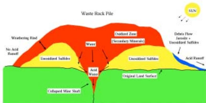
**The Life Cycle of Acid Mine Drainage**
