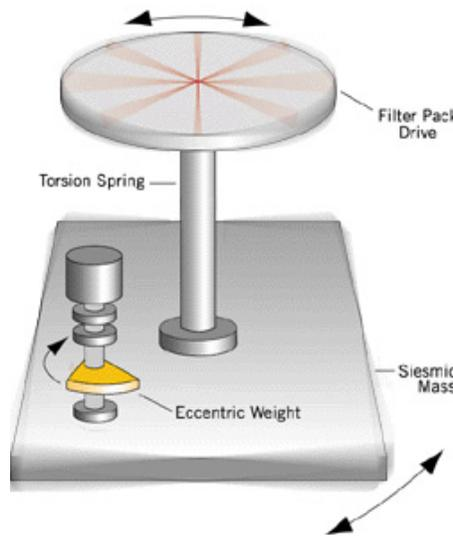
**An eccentric weight induces a wobble that resonates at about 50 Hz giving vibration to the Filter Pack above**
